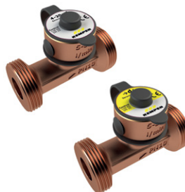
CONTROL-PLUS flow and temperature measuring valve, Figure 138 4G/BMS version Figure 138 6G To precisely determine and adjust volume flows in drinking water systems. Sensor housing with low pressure loss; min. flow velocity 0.2 m/s; max. flow velocity 2.5 m/s; temperature measurement range 0–100°C.
